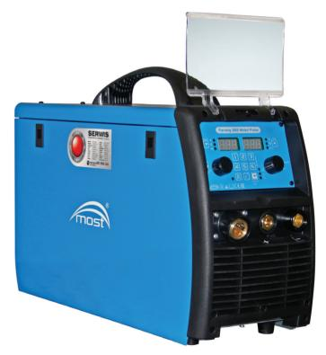
Simple and modern design of control panel. Parameters setup is performed by means of two multifunctional knobs. LCD shows parameter values during setting adjustments and real-time values during work performance. The LEDs next to the LCD informs which parameter is presented and what is the used unit: A, V or s. It is possible to save up to 6 personalized programmes entered to memory with buttons from 1 to 6.
