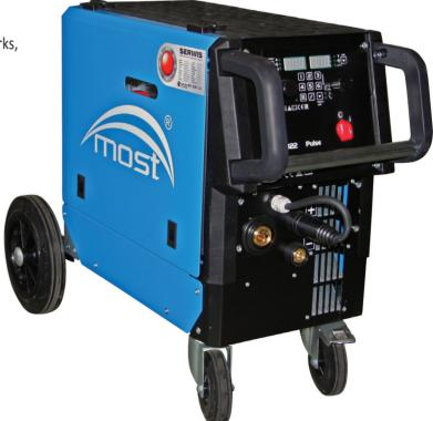
Simple and modern design of control panel. Parameters setup is performed by means of two multifunctional knobs. LCD shows parameter values during setting adjustments and real-time values during work performance. The LEDs next to the LCD informs which parameter is presented and what is the used unit: A, V or s. It is possible to save up to 6 personalized programmes entered to memory with buttons from 1 to 6.
