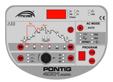
TIG DC welding is performed with a direct or pulsating current of up to 3000 Hz. Additional settings improving the weld quality or welding speed are available for TIG AC aluminium welding with alternate current. MMA method offers VRD safety function for reducing idling voltage to 12 V.
